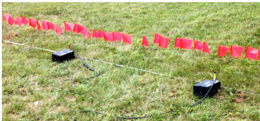
Figure 5.3. Collecting CMP data where the transmitting and receiving antenna are moved apart in steps, with one trace collected every distance of separation. Source: the author.
