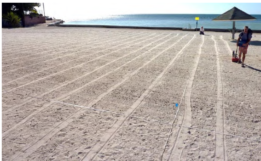
Figure 3.5. Collecting GPR reflection profiles in transects a meter apart, with tracks showing the mostly parallel lines along which the antennas were moved, on a beach in Key West, Florida. Source: the author.
