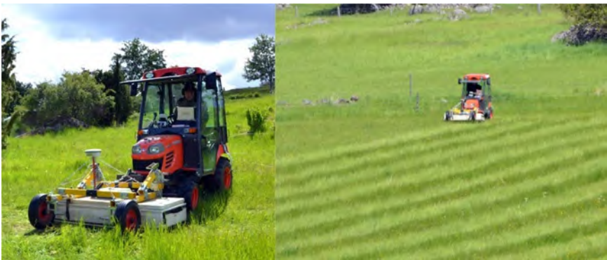
Figure 3.8. An antenna array system moved by a farm tractor in Birka, Sweden. Here seventeen 400 MHz antennas are in the white box, collecting 16 traces spaced 8 cm apart in “swaths” that are about 140 cm wide. Courtesy of Ewe and Immo Trinks.
