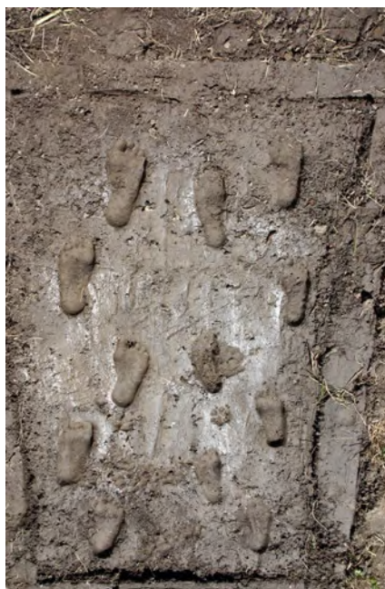
Figure 7.32. Human footprints placed in mud to simulate the Laetoli prints in Tanzania. This model was left to dry in the sun and then covered with sand for testing with very high-frequency antennas. Source: the author.
