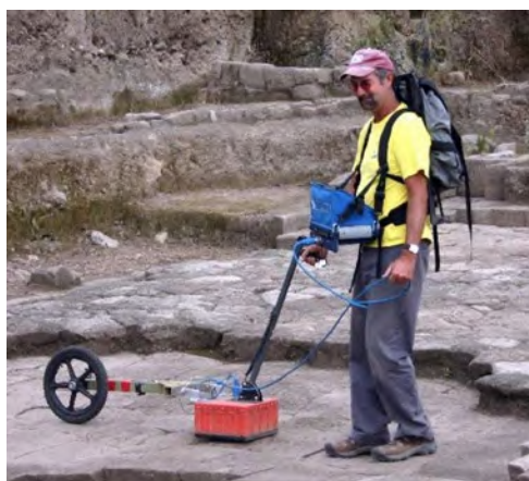
Figure 3.6. Collecting 400 MHz using a system supported in a backpack with an attached survey wheel for distance measurement, on an Inca floor in Ecuador. Source: the author.
