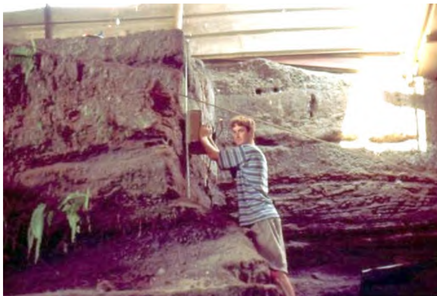
Figure 5.6. Collecting transillumination data with one receiving on a vertical face of volcanic ash at Ceren, El Salvador. The transmitting antenna is on a parallel exposure off camera to the left. Source: the author.
