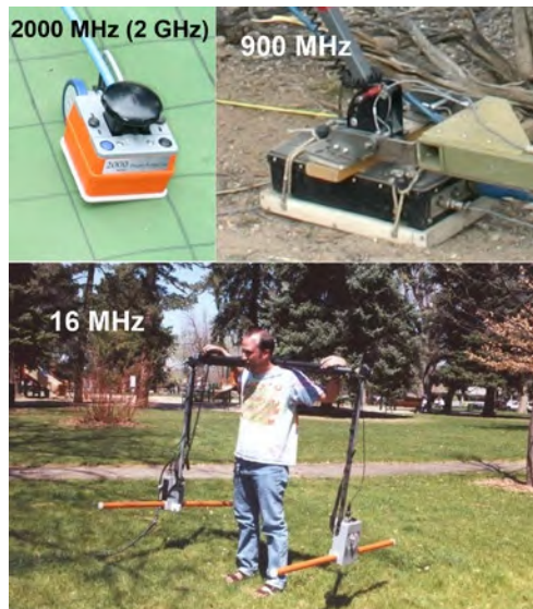
Figure 3.17. Antennas of various frequencies from the 2 GHz “palm” antenna to the 16 MHz very low frequency antenna, with a more normal-sized 900 MHz antenna. Source: the author.
