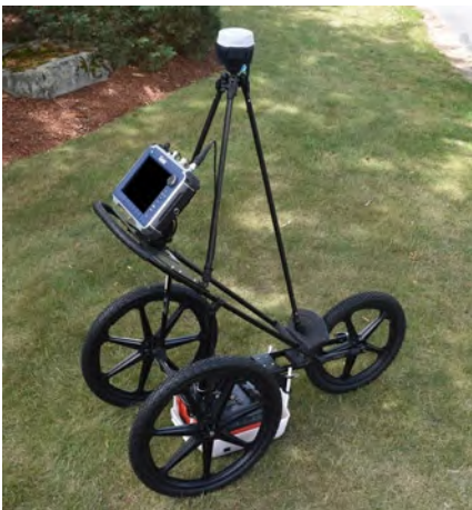
Figure 2.3. A GSSI SIR-4000 recording system with 400 MHz antennas on a survey cart with an attached RTK GPS antenna for location data. Courtesy of GSSI Inc.
