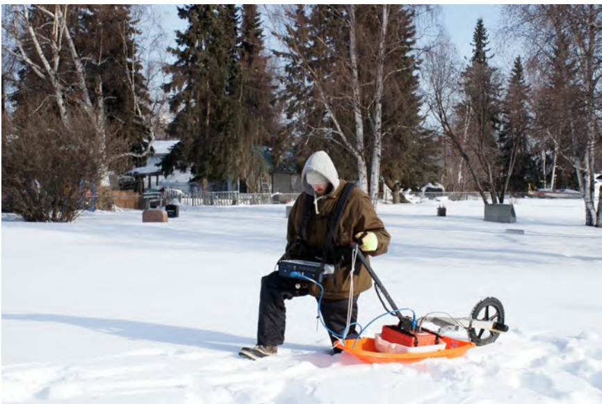
Figure 3.29. Collecting GPR data in snow in Alaska. Source: the author.
